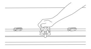
A cutting guide fitted with a diamond tip tool is recommended.
