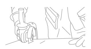
The slabs can also be cut with a dry saw or wet saw with a diamond wheel cutter.
