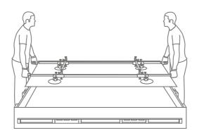
Handling the slabs on the floor can be managed with the aid of a frame fitted with suction cups to make the slabs more stable.
