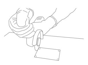
For L-shaped cuts or cuts inside the slab, holes should be bored at the vertices to prevent the blade of the cutting disk damaging the surface.
