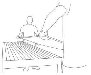
Where possible, mechanical lifting systems should be used for delivering slabs above the ground floor.
