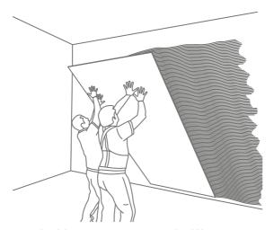
Once the slab is in position, excess air should be removed completely by tapping it either manually or mechanically using the appropriate trowel, starting from the centre and moving out towards the sides.
